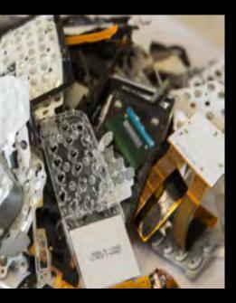
Mobile phones are composed of about 40% plastic compounds. The case of a mobile phone is typically made of PC/ABS plastic, a mix of polycarbonate (PC) and acrylonitrile butadiene styrene (ABS). The case of the charging station is typically made of polycarbonate
