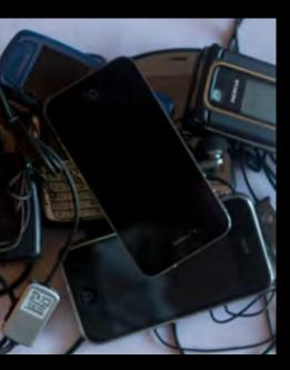
A mobile phone is typically composed of about 40% of plastic, 32% of non-ferrous metal, 20% of glass and ceramics, 3% of ferrous metal and 5% other. Mobile phones differ from manufacturer to manufacturer and from model to model. Consequently, the substances used in any mobile phone will be somewhat different from the substances used in another.
